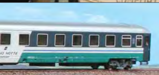
Set ICN composto da due carrozze a cuccette Tipo UIC-X Treno Notte Comfort (T4) con porte blu e una carrozza letti Tipo MU. Set ICN composed by two Type UIC-X "Treno Notte Comfort" couchette cars (T4) with blue doors and one Type MU sleeping car. Set ICN bestehend aus zwei UIC-X Liegewagen der FS "Treno Notte Comfort" (T4) und einem MU Schlafwagen.
