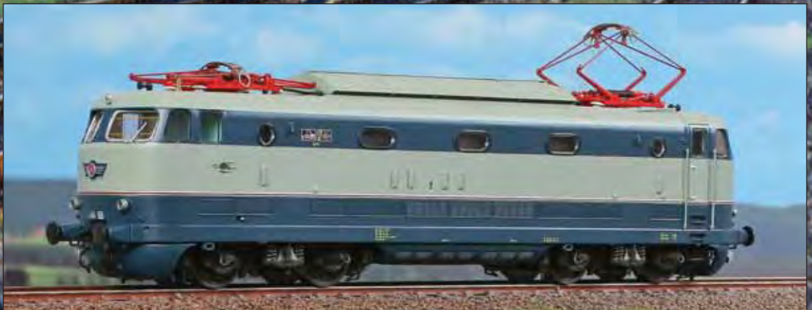
Locomotiva elettrica E.444.093 di II serie, senza baffo rosso, con modanature. Electric locomotive E.444.093, 2nd series, without red plank and with mouldings. Elektr locomotive E.444.093, ohne rote Front und mit Zierleisten.
