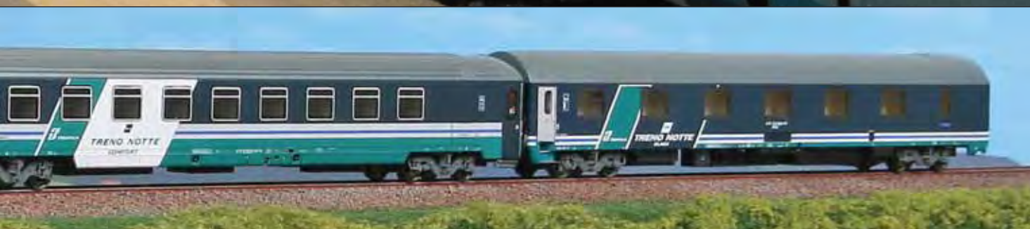
Set ICN composto da due carrozze a cuccette Tipo UIC-X Treno Notte Comfort (T4) con porte blu e una carrozza letti Tipo MU. Set ICN composed by two Type UIC-X "Treno Notte Comfort" couchette cars (T4) with blue doors and one Type MU sleeping car. Set ICN bestehend aus zwei UIC-X Liegewagen der FS "Treno Notte Comfort" (T4) und einem MU Schlafwagen.
